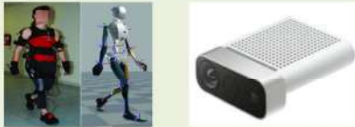
< Figure1. Motion capture suit(좌) 및 Azure Kinect(우) >
